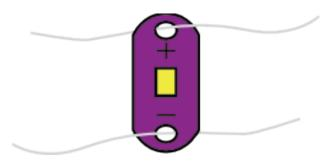
After making sure that the LEDs are correctly threaded then attach each end to one of the screws, make sure not to cross the threads. When tying off the threads draw the thread tight, but not so tight that you will have a hard time moving the LEDs up and down. Also leave a good three to four inches hanging off each nail at the end you intend to connect to the power source.
