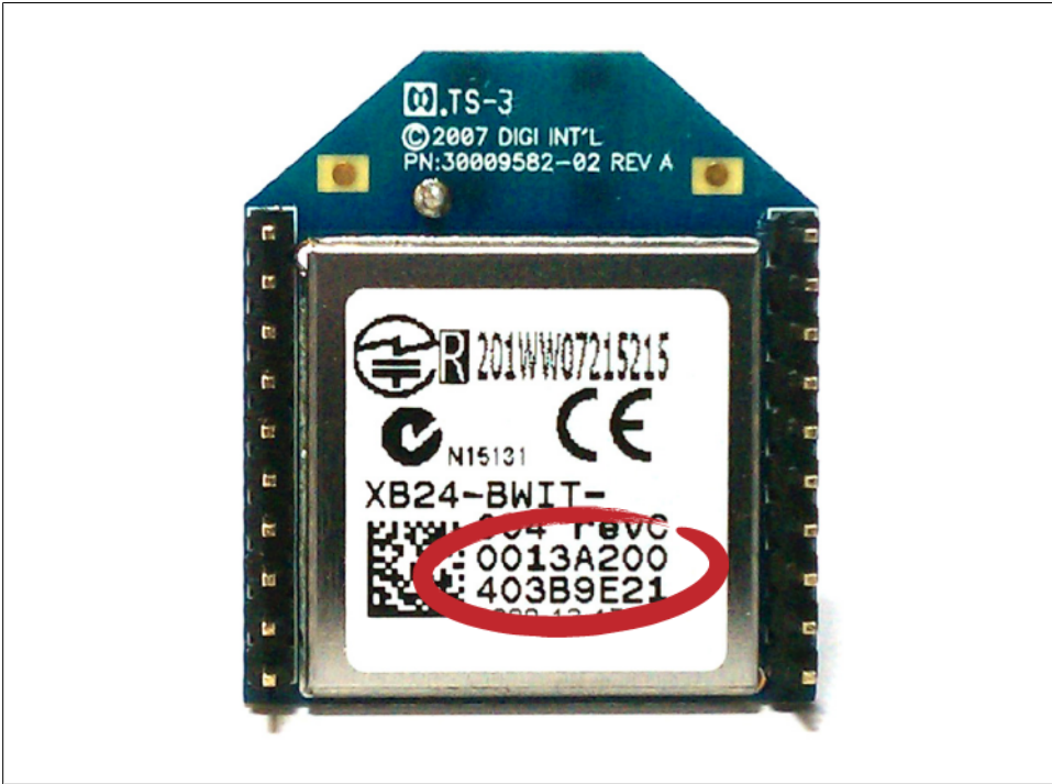
Figure 2-22. Back of XBee showing 64-bit address
