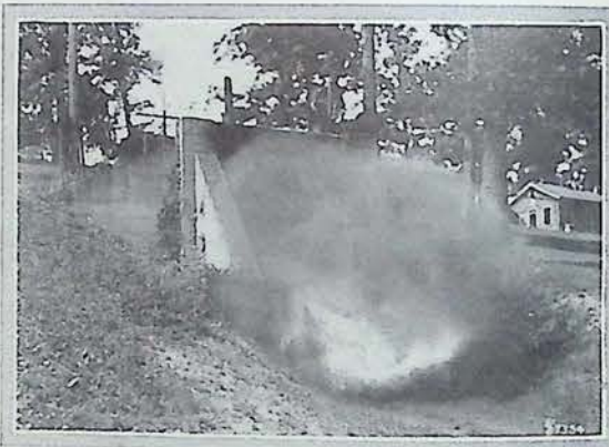
Flame and smoke emerging from portal of Experimental Mine, following a test explosion.
