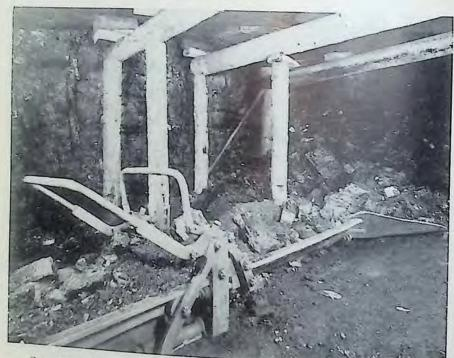
Second development of the Duckbill—the substitution of grip blocks for rack and pinion.
